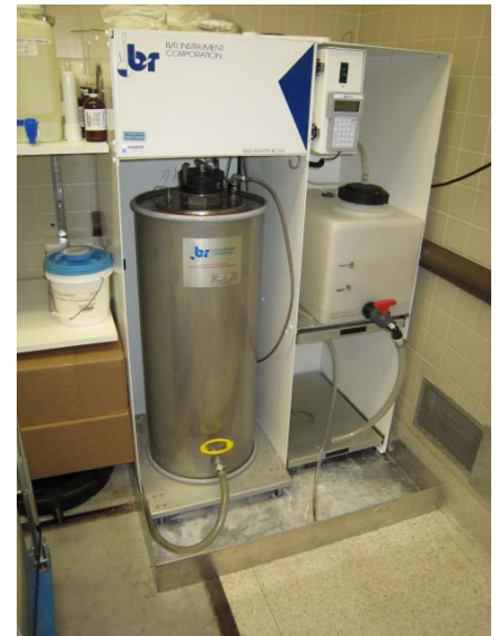
The formalin recycling unit program is a cost-effective alternative to hazardous waste disposal of used formalin or chemically neutralizing formalin prior to sewer disposal.
