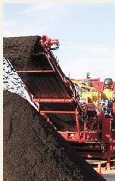
Ground up roof shingles find new life as an ingredient in asphalt pavement.
