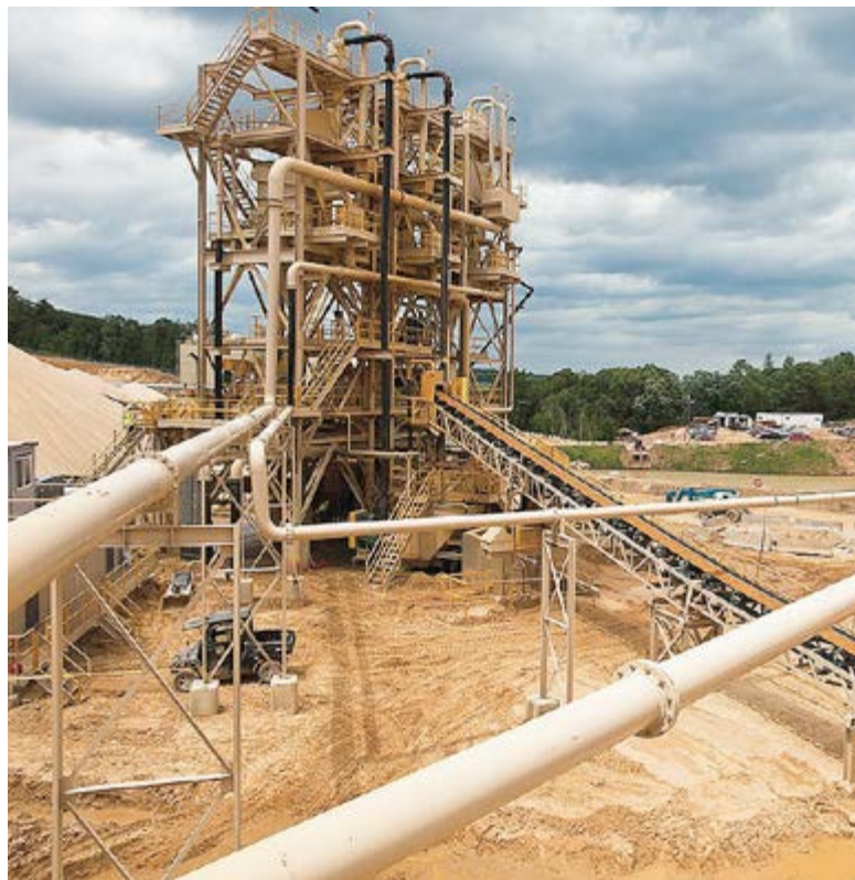
Photo by Lukas Keapproth/Wisconsin Center for Investigative Journalism A conveyor moves crushed sand to be washed and sorted by grain size at the Preferred Sands plant in Blair, Wis. in Trempealeau County.
