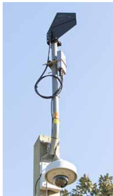
A pole-mounted “super Wi-Fi” radio transmits security-camera images from a New Hanover County, N.C. park.
