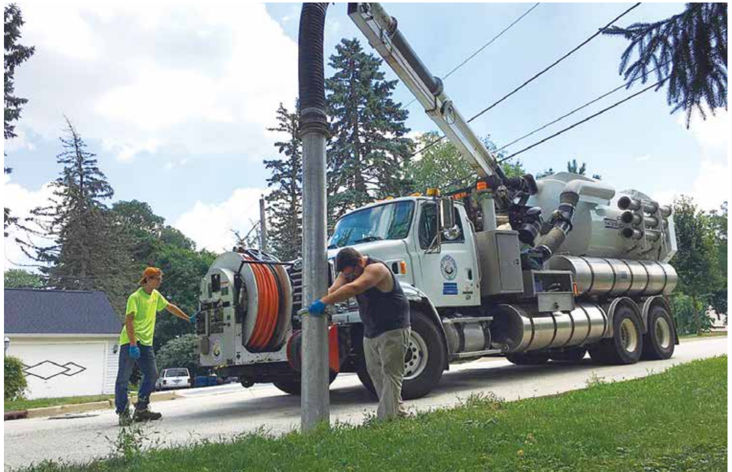
DuPage County Stormwater Management's Shared Services Senior Maintenance Worker Tom Klasen works to clean the storm sewer system in the Village of Itasca, Ill. Photo courtesy DuPage County
