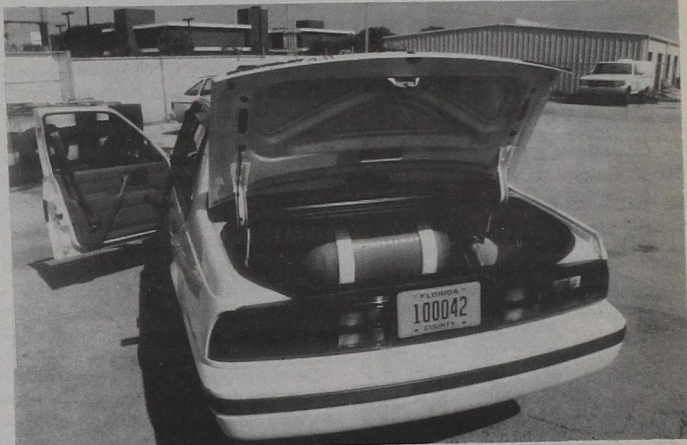
A Broward County, Fla. public works vehicle that runs on natural gas — the tank is located in the trunk.
