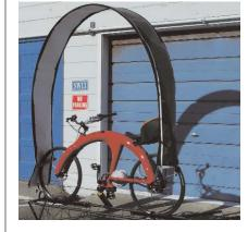
features proprietary electric beltdrive, in-wheel infinitely variable transmission, on-the-fly seat and handlebar adjustments, and a patentpending aluminum monocoque that houses battery packs, vital electronics,
