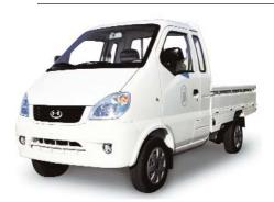
changes in the Federal Air Bag Standards, but should be on sale in California in early 2009. These revolutionary cars have a top speed of 25 mph, range of 40-50 miles, cargo capacity of 41 cubic feet, and capacity for four occupants. The truck has a top speed of 25 mph, range of 50-60 miles, 3000 lbs. GVWR, cargo area of 75" x 54" x 11", and charging time of four to six hours. www.milesev.com
