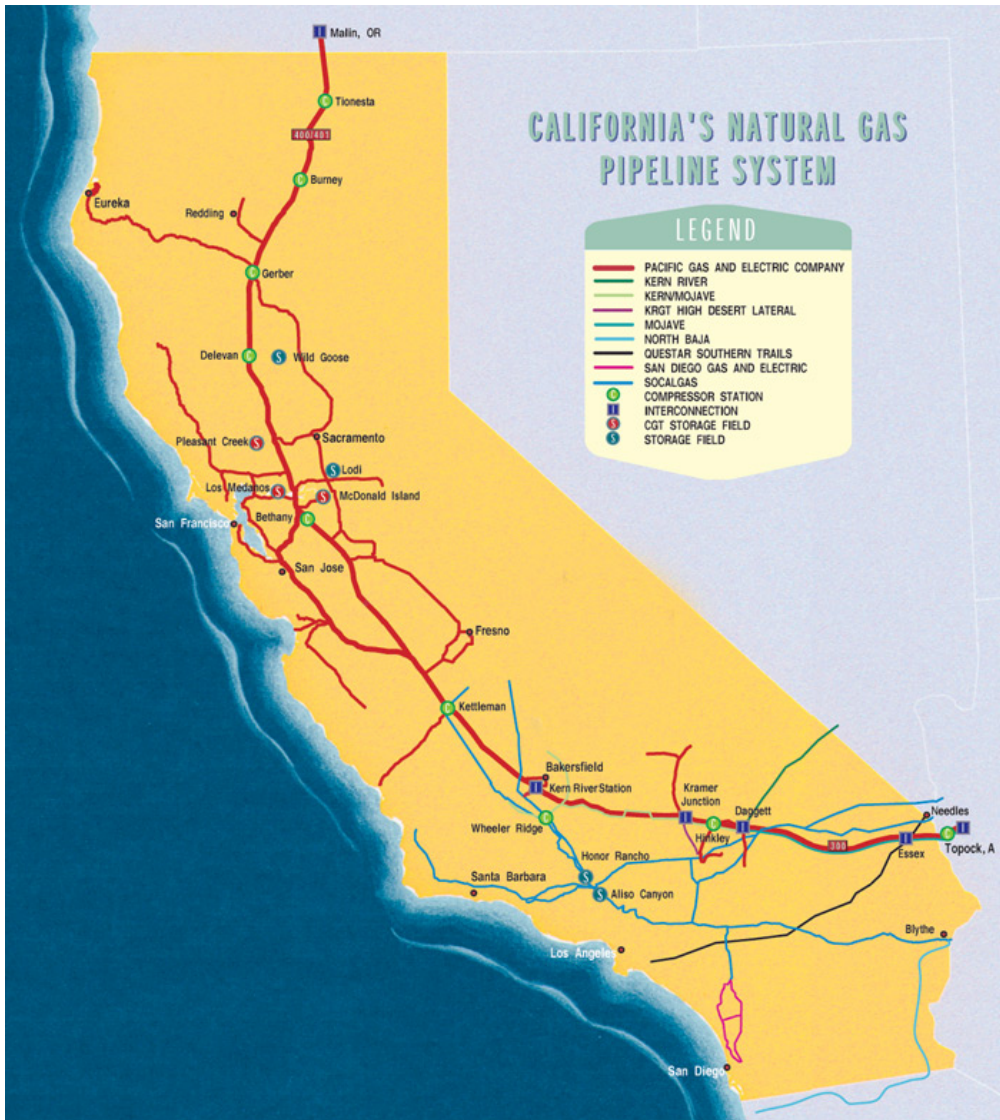
Figure 7: Diagram of the natural gas pipelines within California that supplies Humboldt County.
